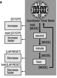
NOTE: If NO INPUT for 1 minute during the setup, the display will default to the Countdown Timer Mode
